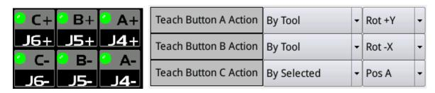
Each of the three ABC keys can be set to its operation mode, which is set by the login authority above the machine maker ID.
