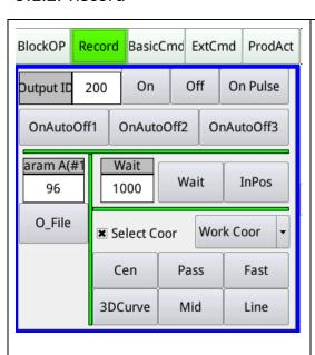
The recording function is mainly for the convenience of quickly teaching a motion path, so only a few path commands and output control commands are placed on the screen.
