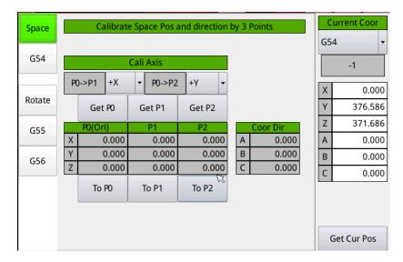
Mathematically, we can determine a coordinate system through three point positions, where:
