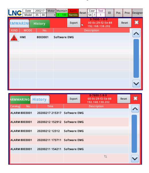
Note 1: The user-defined alarm warning exists in ReconTool/file/language/UserAlarm\_0000.str, which can be downloaded and edited, and then uploaded to overwrite the original file. The alarm range is from R29000.00 to R29049.31, and the warning range is from R29050.00 to R29099.31.
