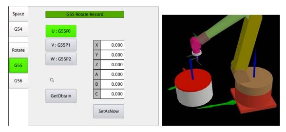
The system provides up to three rotating coordinate systems corresponding to up to three additional axes.
