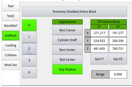
The system provides up to five groups  $(0 \sim 4)$  of sharp point range settings, which can be switched in manual mode or dynamically switched during automatic program operation.
