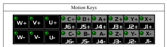
When the button light is on, it means that the button will work when pressed. If it is not lit, it will not work.
