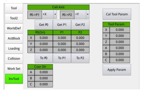
The calibration method is similar to that of the coordinate series, except that the original workpiece is external and is clamped at the end of the robot.
