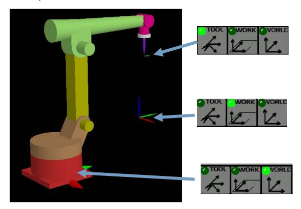
Joint Coordinate System: Defines the decision based on the direction in which the joint rotates.
