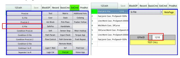
Note: There is also a command called G file in the basic command, which can pass parameters to G file. The G code exported by the above method cannot receive the parameters passed in when calling from the upper layer. You can achieve the effect of receiving the parameters by writing the G code by yourself and running according to the content of the parameters.
