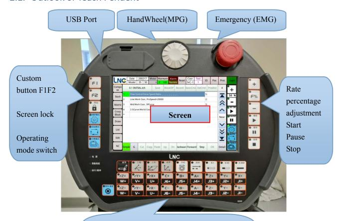
Manual operating coordinate system selection, handwheel operation switching rate multiplier (x1, x10, x100), axial key (J1~J9), System reset button
