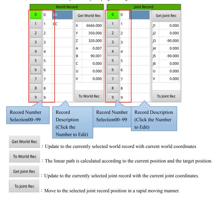
Note 1: The point record can be used as a coordinate system in addition to the point of operation.
