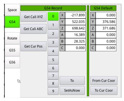
This system provides 10 sets of coordinate system records and a set of coordinate systems that are preset to be brought in at startup to meet the needs of multiple machining areas.
