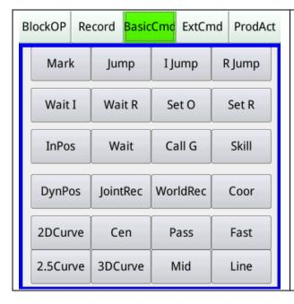
The basic commands include the flow control type, waiting type, state setting type, and the motion command.
