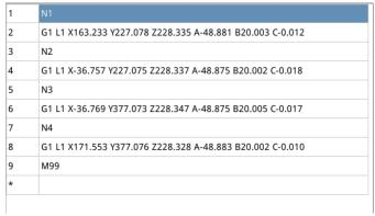
Note 2: If the macro instructions of this system are familiar, you can also directly edit the page with NC, or write directly with a PC's text editor to generate an O file and use it directly, to save the process of exporting again.
