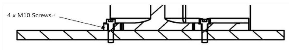
Figure 2.17 Robot mounted directly on the ground
