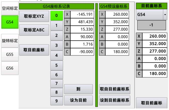
$\underline{ \text{Rule: The moving direction of the conveyor belt is the $X$+ direction of the working coordinate system.} \\$
