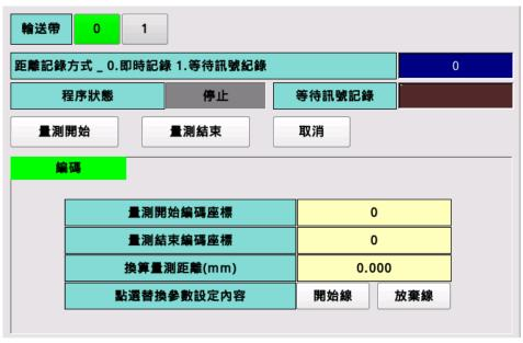
After the measurement starts, record the coordinates of the measurement start code and the coordinates of the measurement end code according to the recording mode, and convert the distance moved,
