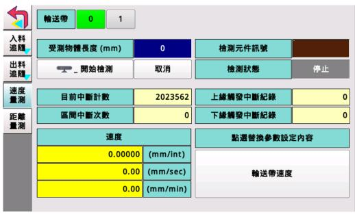
The system will calculate the moving speed of the conveyor belt according to the set object length and detect the object moving on the conveyor belt. The calculated result can determine whether to replace the current speed reference value according to the situation.
