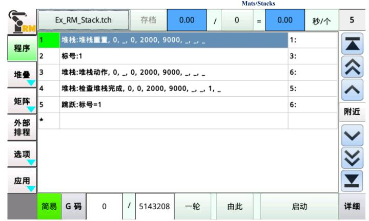
If you want to clear the current stack operation information when the program restarts, you need to use the stack reset instruction with the label and jump mode, as shown in the figure above. (If you do not need to clear it, you can leave it out)
