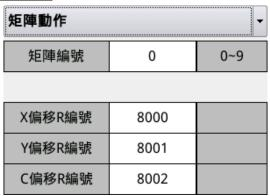
Set the matrix number setting and the R buffer address with a uniform offset.
