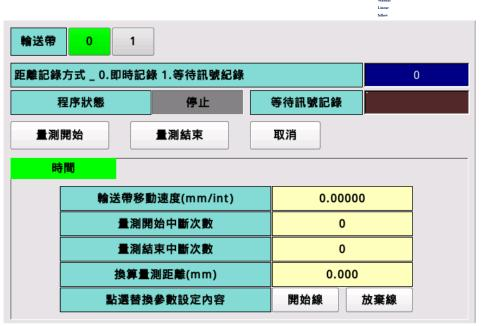
After the measurement starts, it will refer to the moving speed of the conveyor belt and record it until the end of the measurement, and convert the distance moved. You can use the shortcut key to replace the Settings of the start line or the abandon line.
