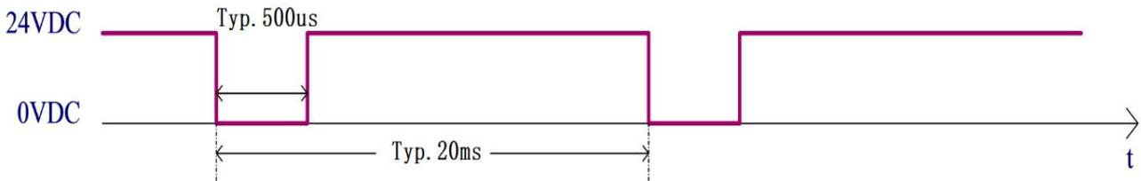
**Figure 7 Security Input Sequence Diagram**
