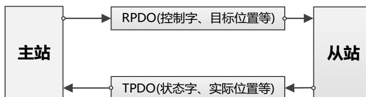
Figure 6-2-2 PDO transmission model
