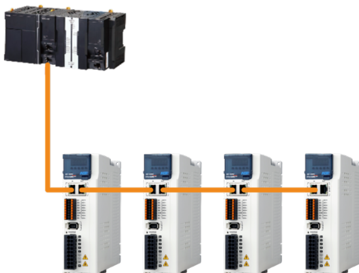
Figure 6.1.1 - Schematic diagram of the EtherCAT network
