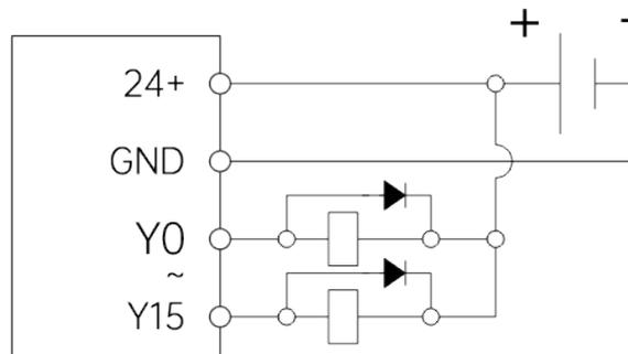
Figure 3-6: DO output NPN type wiring diagram
