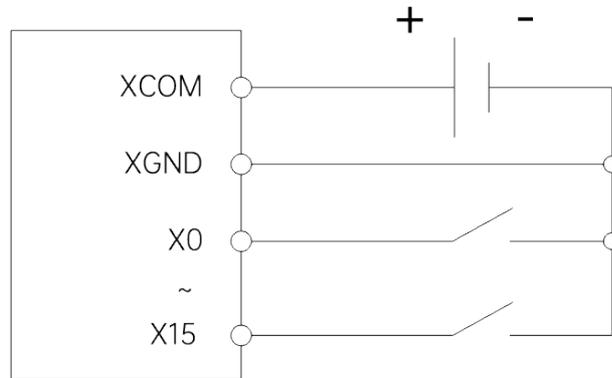
Figure 2 -4: DI active input NPN type wiring diagram
