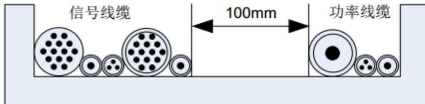
Figure 5-9 Cabling with different levels of cables
