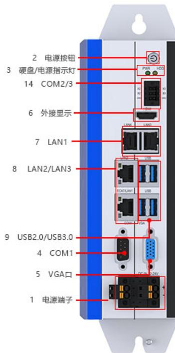
Figure 3-3 HMC-G310/G320/G360 controller appearance
