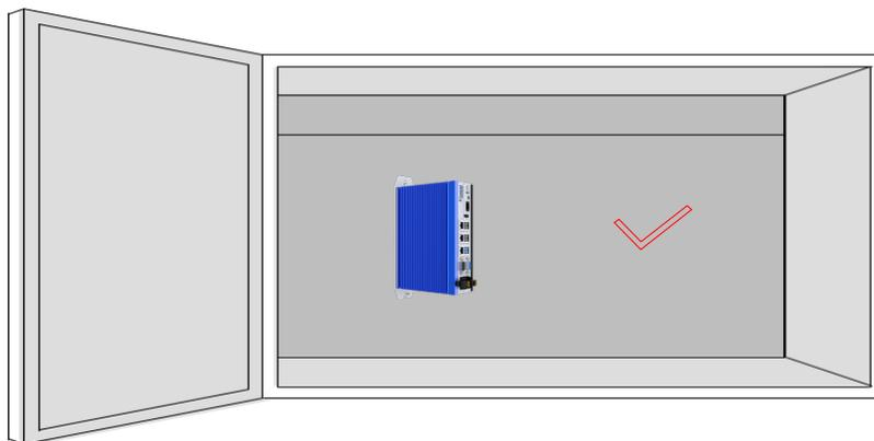
Figure 5-2 Mounting direction
