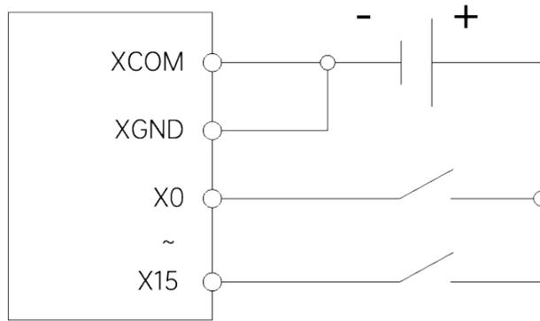
Figure 3-3: DI active input PNP type wiring diagram
