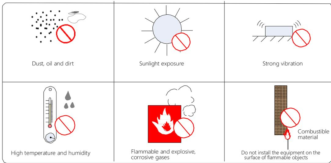
Figure 5-1 Installation environment requirements
