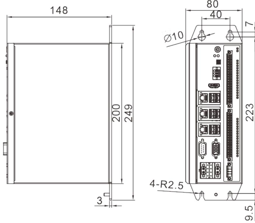
Figure 3-8: HMC-G301-2000 controller exterior dimensions (unit:mm)
