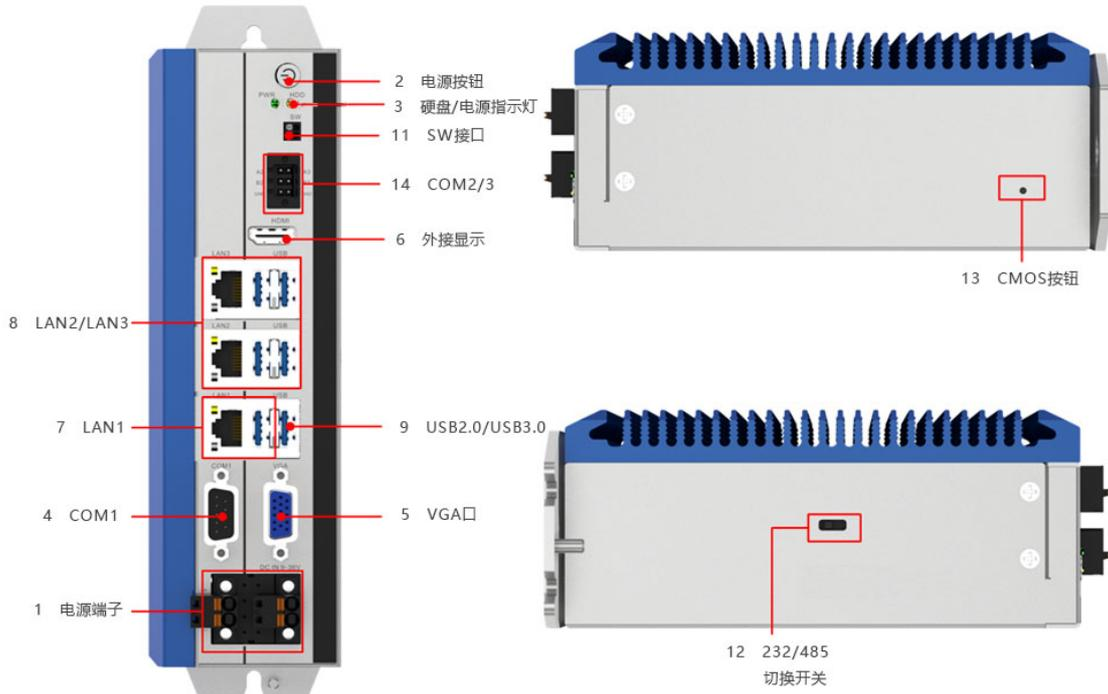
Figure 3-1 HMC-G300-2000 controller appearance
