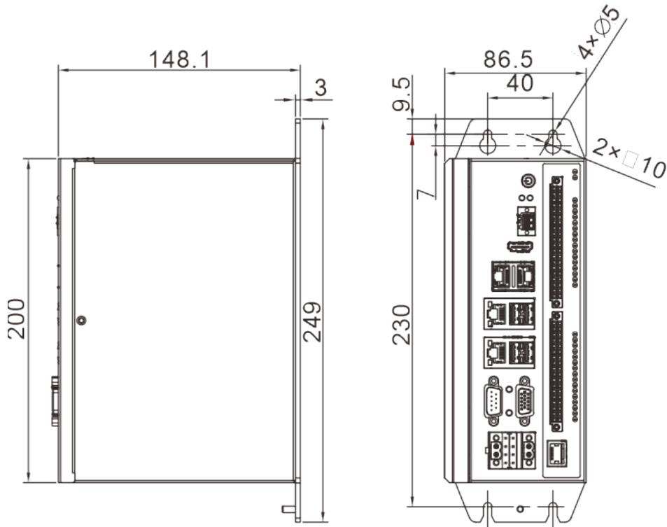
Figure 3-10: HMC-G311/G321/G361 controller exterior dimensions (unit:mm)
