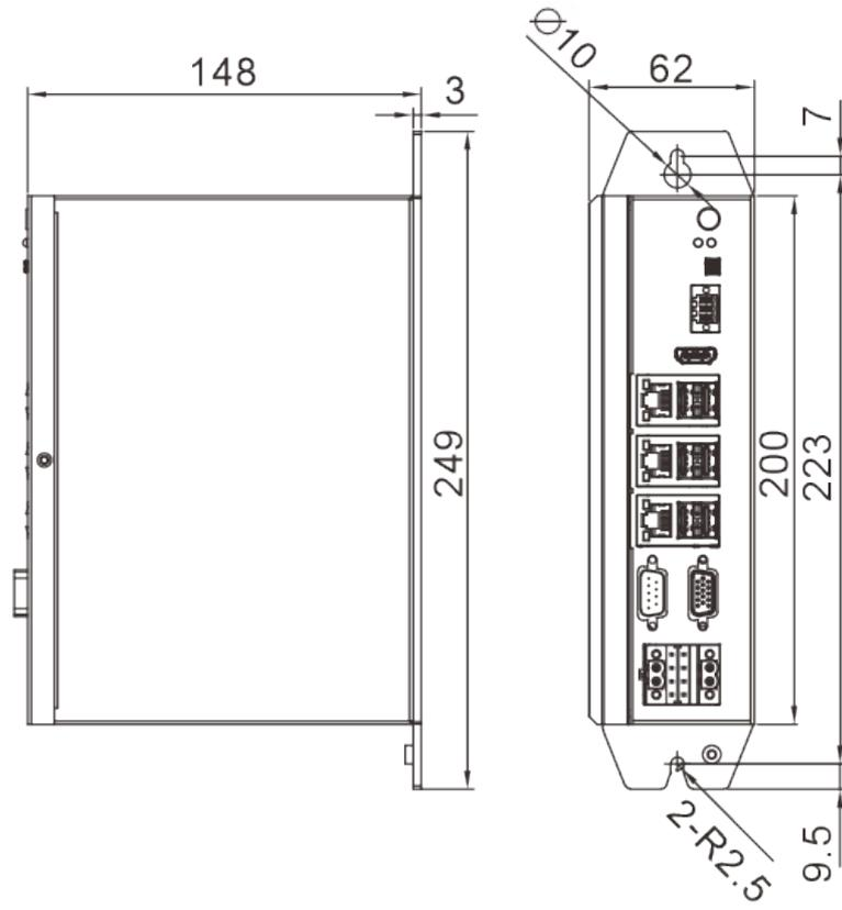
Figure 3-7: HMC-G300-2000 controller exterior dimensions (unit:mm)
