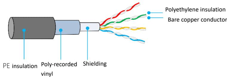
Figure 5-8 Communication cable shield diagram
