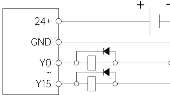
Figure 3-5: DO output PNP type wiring diagram
