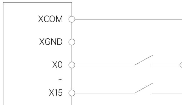
Figure 1 : DI passive input wiring diagram
