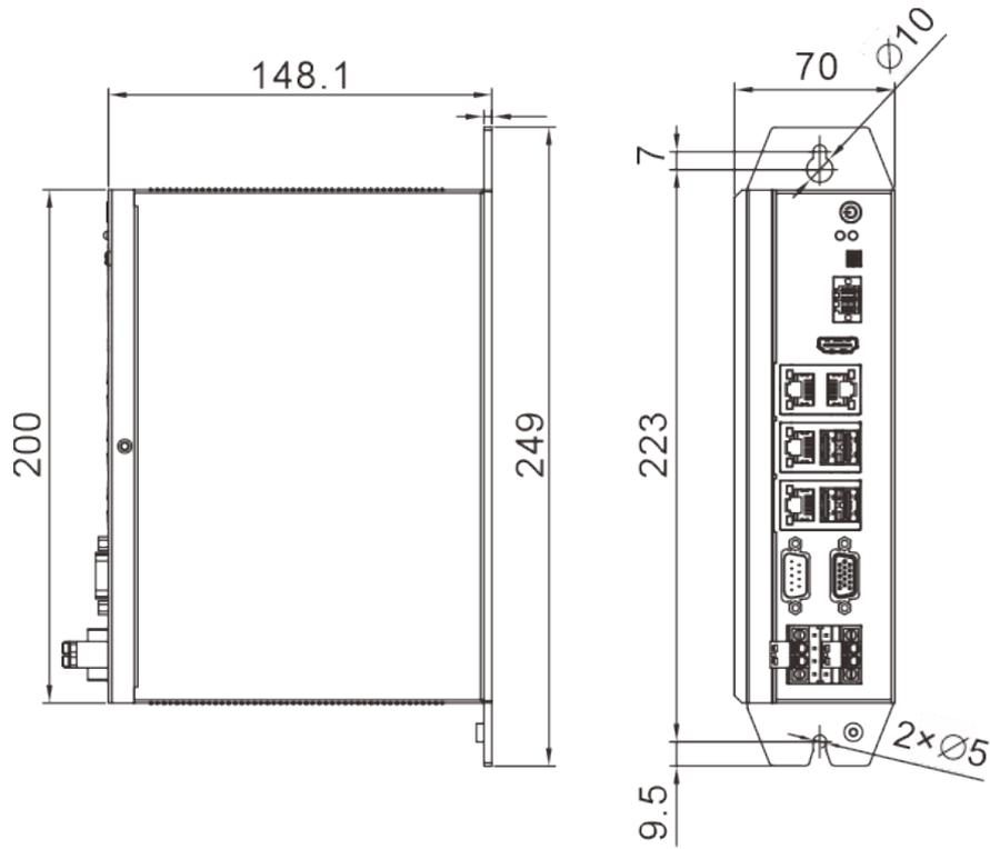
Figure 3-9: HMC-G310/G320/G360 controller exterior dimensions (unit:mm)
