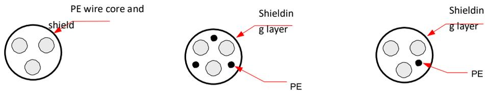
Figure 5-6 Schematic diagram of symmetrical shielded cable
